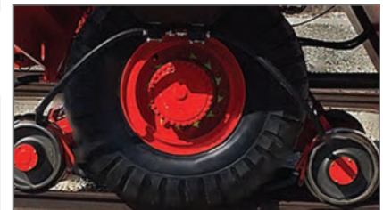
Patented rail guidance system: two independent drive wheel trucks supported on rotating bearing with eight 16" AAR profile guide wheels. ABS & traction assist provide more control while reducing maintenance costs.
