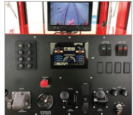
180-degree rotating console with a multifunction display. Dual four-way air suspension seats for operation from either side of cab when in rail mode.
