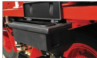
Pull out sander boxes with wide mouth lids for easy loading. Air activated sanders for smooth dispensing.
