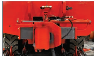
Wide range AAR sliding couplers are air released and hydraulically positioned to improve pulling performance on curves and grades.
