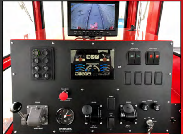
180 degree rotating console with multifunction display. Dual four-way air suspension seats for operation from either side of cab when in rail mode.
