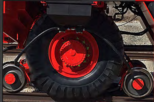
Two independent drive wheel trucks supported on rotating bearings with eight 16" AAR profile guide wheels. ABS & traction assist provide more control while reducing maintenance costs.
