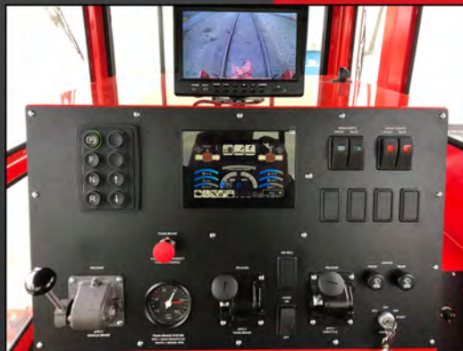
180 degree console with color multifunction display. Dual four way air suspension operator seats for either side on-rail operator control.
