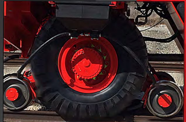
Patented rail guidance system: two independent drive wheel trucks supported on rotating bearings with eight 16" AAR profile guide wheels. ABS & traction assist provide more control while reducing maintenance costs.
