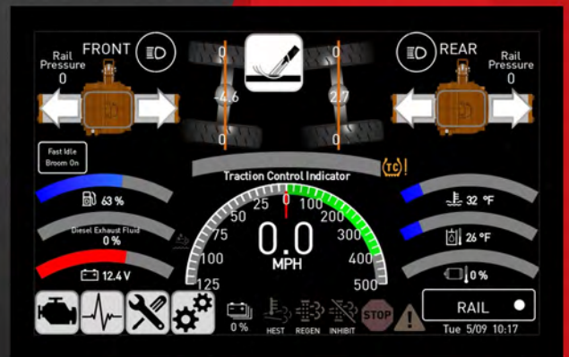
In dash multi-functional digital display module with push button controls on a 180 degree rotating operator console.
