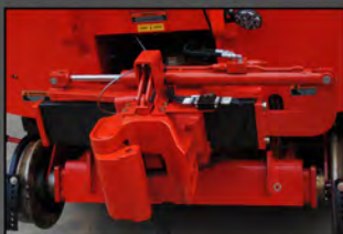
Wide range AAR sliding couplers are air released and hydraulically positioned to improve pulling performance on curves and grades.
