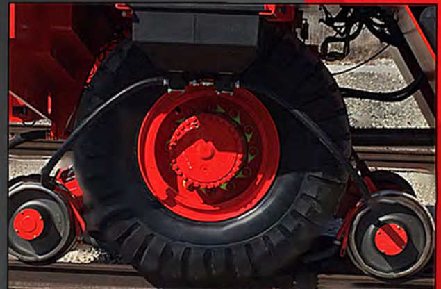
Patented rail guidance system: two independent drive wheel trucks supported on rotating bearings with eight 16" AAR profile guide wheels. ABS and traction assist provide more control while reducing maintenance costs.
