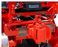
Wide range AAR sliding couplers are air released and hydraulically positioned to improve pulling performance on curves and grades.
