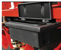
Pull out sander boxes with wide mouth lids for easy loading. Air activated sanders for smooth dispensing.
