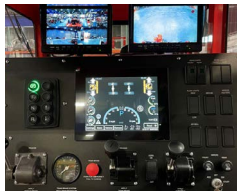
180-degree rotating console with a multifunction display. Dual four-way air suspension seats for operation from either side of cab when in rail mode.
