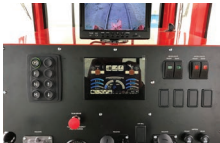
180-degree rotating console with a multifunction display. Dual four-way air suspension seats for operation from either side of cab when in rail mode.
