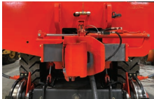
Wide range AAR sliding couplers are air released and hydraulically positioned to improve pulling performance on curves and grades.
