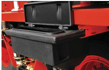
Pull out sander boxes with wide mouth lids for easy loading. Air activated sanders for smooth dispensing.
