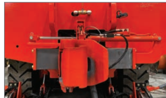
Wide range AAR sliding couplers are air released and hydraulically positioned to improve pulling performance on curves and grades.
