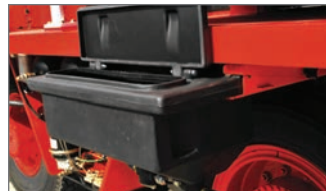
Pull out sander boxes with wide mouth lids for easy loading. Air activated sanders for smooth dispensing.
