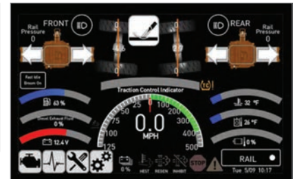
In dash multi-functional digital display module with push button controls on a 180 degree rotating operator console.
