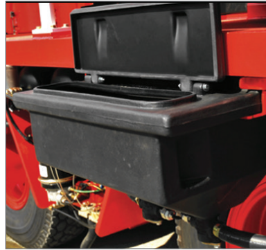
Pull out sander boxes with wide mouth lids for easy loading. Air activated sanders for smooth dispensing.
